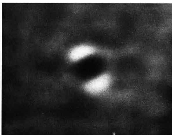
Fig. 1. Light optical correlation functions of electron micrographs (carbon foil, Elmiskop 101, M = 510\,000 ), a) autocorrelation function at overfocus ( \Delta z = 1000\text{ \AA} ), b) autocorrelation function at underfocus ( \Delta z = -500\text{ \AA} ), c) cross-correlation function of two micrographs at overfocuse and underfocus (contrast reversal).
